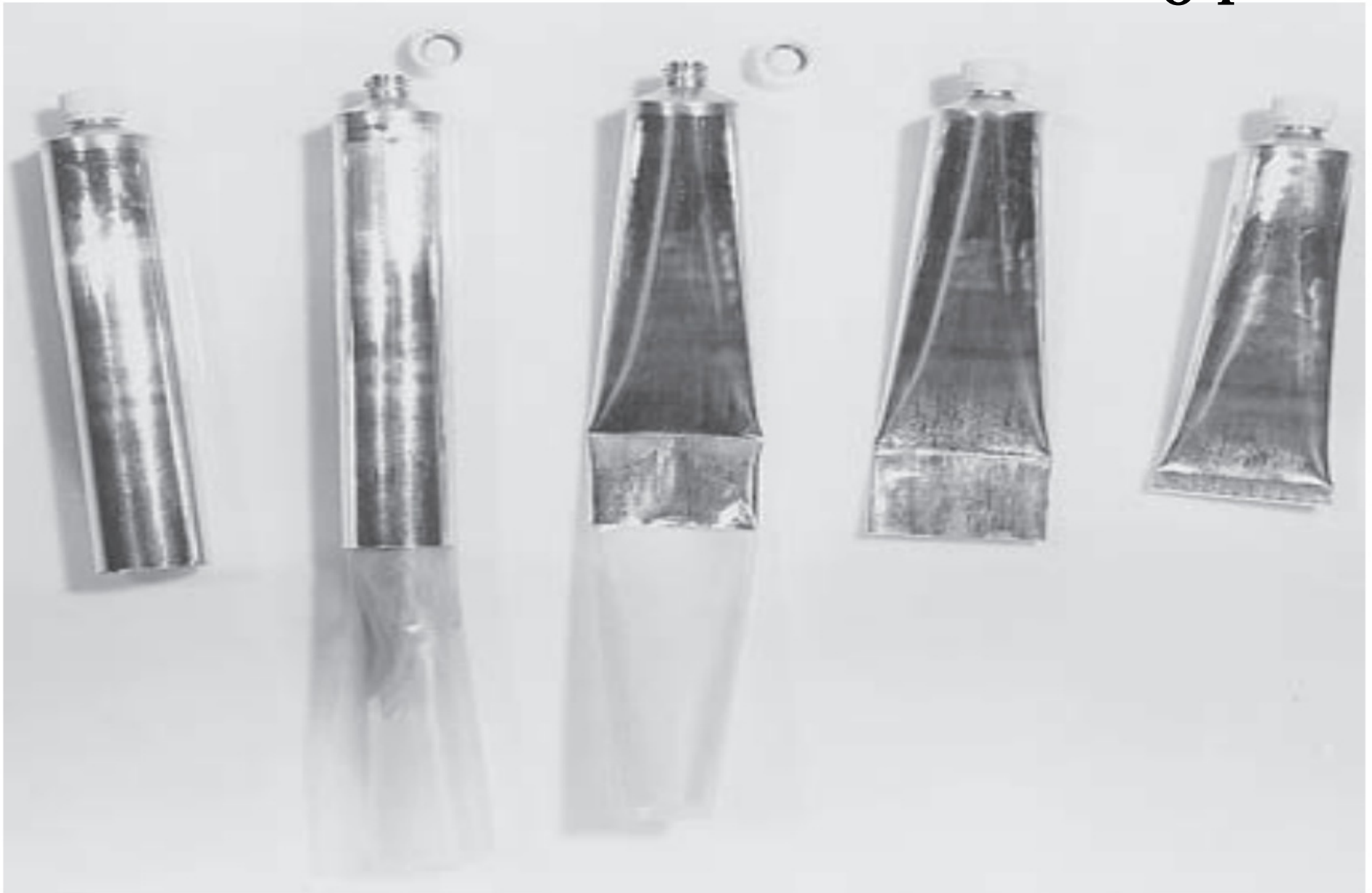
FIGURE 10.7 Steps in the manual filling of ointment tubes.
