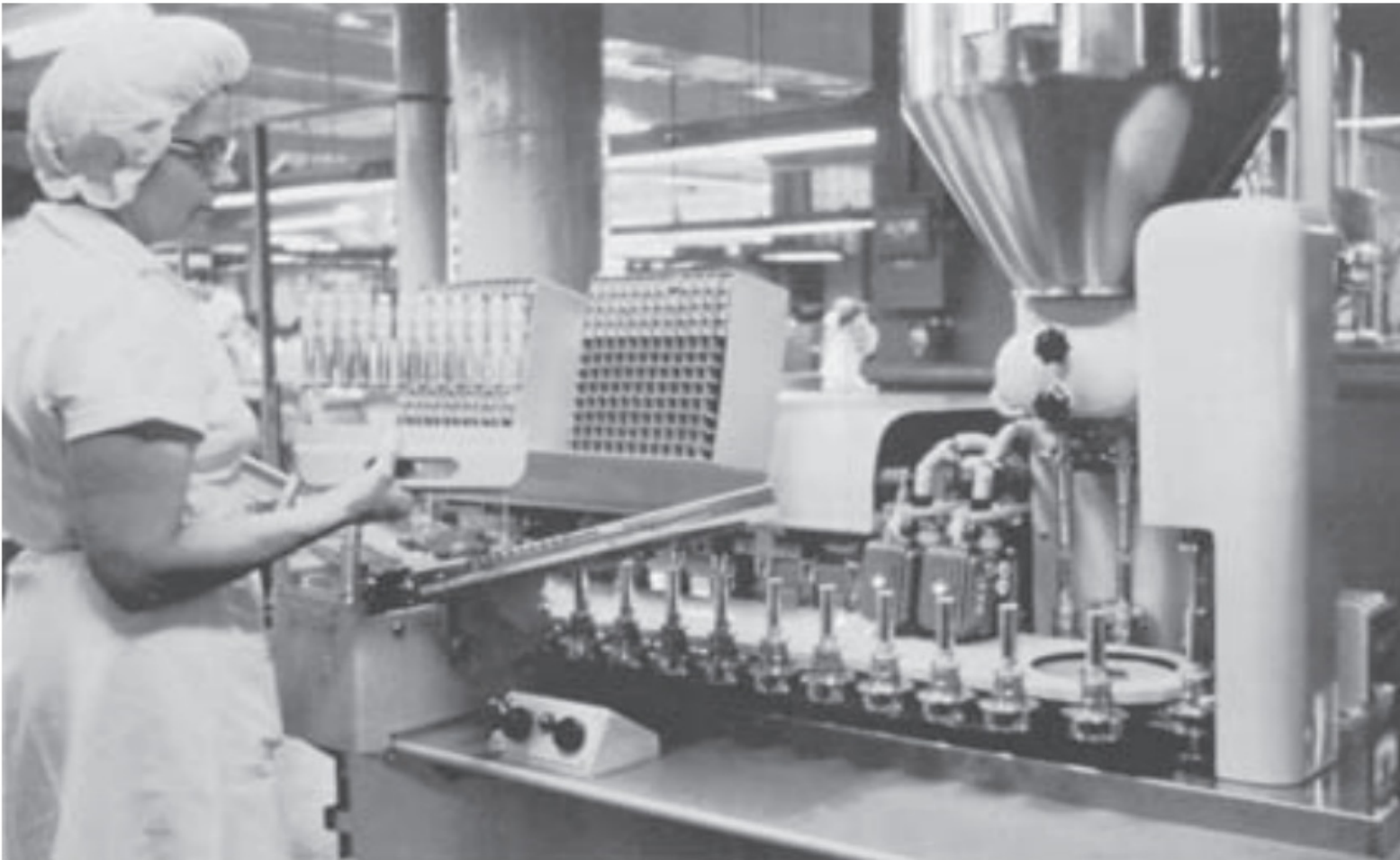
FIGURE 10.6 Arenco tube-filling machine automatically fills 125 tubes a minute with proper amount, tightens cap, orients each tube by electric eye so that label faces forward, then closes and crimps the end. (Courtesy of Eli Lilly and Company.)
